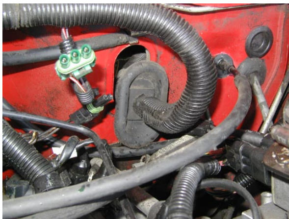
This is the outgoing engine's control trunk to and from the old PCM. It can be removed entirely.
