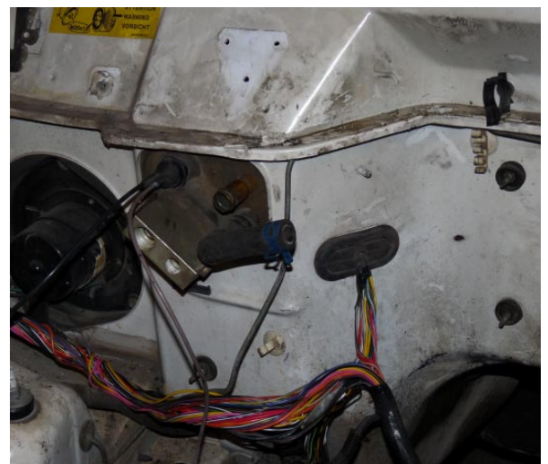
The grommet on the flank of the firewall indentation has the Transmission Control Module circuits. It can be entirely removed and the grommet can be nicely plugged with black RTV silicone.
