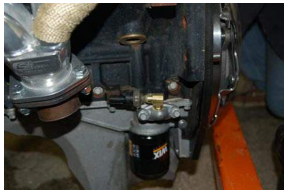
Note the location of the Jeep oil pressure sensor on this Gen. III+ engine (above) and the water temperature sensor (below). It may be necessary to drill and tap as per the threads in your factory or aftermarket sensor.
