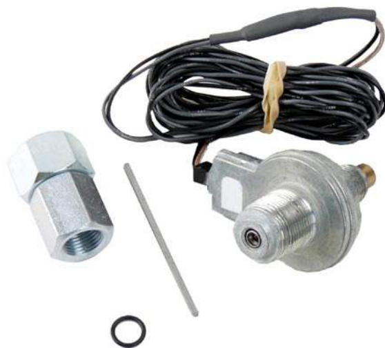
This aftermarket variable reluctance speed signal generator will send a pulsed speed signal to the GM PCM from the transfer case speedometer gear, while allowing for speedometer cable pass-through if you're retaining your factory mechanical speedometer.
