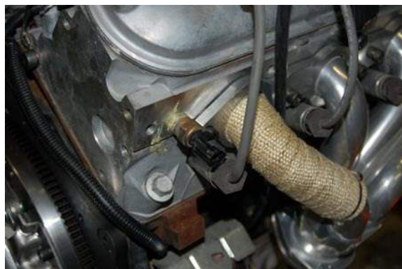
Note the location of the Jeep oil pressure sensor on this Gen. III+ engine (above) and the water temperature sensor (below). It may be necessary to drill and tap as per the threads in your factory or aftermarket sensor.
