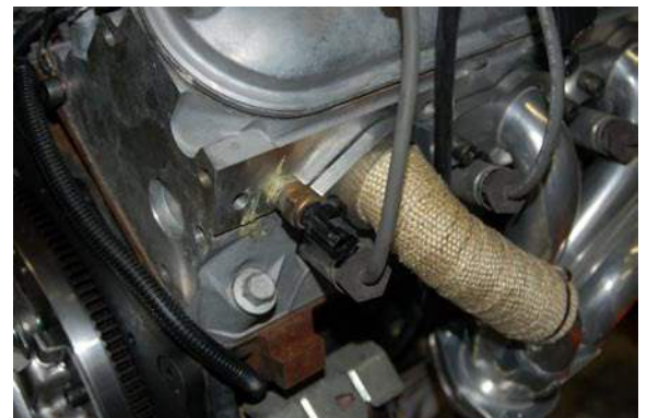
Note the location of the Jeep oil pressure sensor on this Gen. III+ engine (above) and the water temperature sensor (below). It may be necessary to drill and tap as per the threads in your factory or aftermarket sensor.
