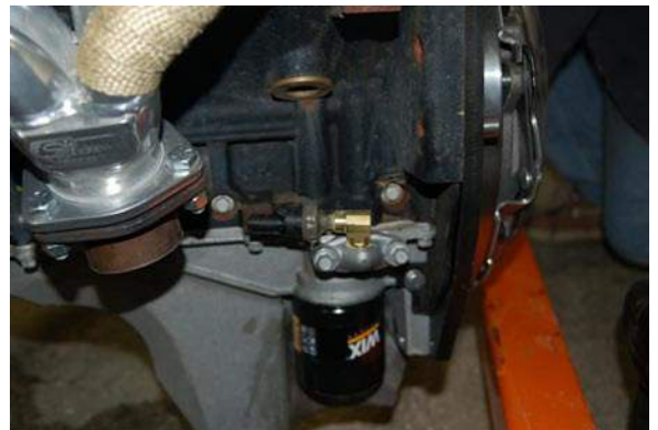
Note the location of the Jeep oil pressure sensor on this Gen. III+ engine (above) and the water temperature sensor (below). It may be necessary to drill and tap as per the threads in your factory or aftermarket sensor.
