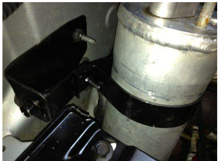
Remove the air conditioning dryer / receiver by detaching the bracket and removing the spring clip.
