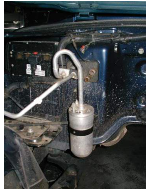
Remove the air conditioning dryer / receiver by detaching the bracket and removing the spring clip.
