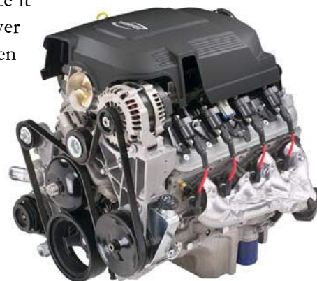
Factory engines such as this 2007 L76 6.0L are as much as 1-1/2" unnecessarily tall with their plastic covers installed.
