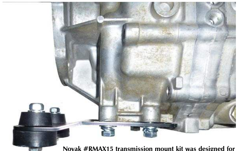
Novak #RMAX15 transmission mount kit was designed for the needs of conversion installers. It can be positioned in a variety of orientation and spacing options.
