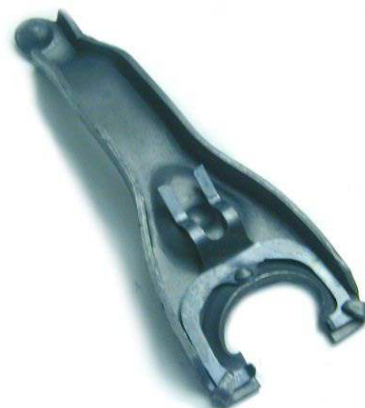
This Chevy release arm is 6.5" long with a ratio of 2.17:1. This will provide proper geometry for the Jeep mechanical release linkage. It is listed at Novak part #RAGM.
