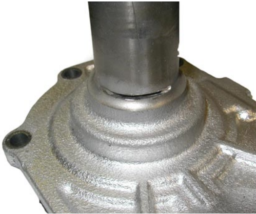
Remove the input bearing retainer and cut the retainer snout / throwout sleeve roughly at this location.
