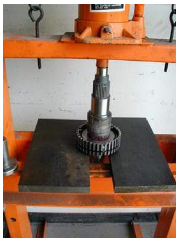
Pressing the 1st-2nd synchronizer hub onto its splines.
