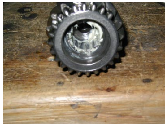
Installing the rollers into the input shaft bore.
