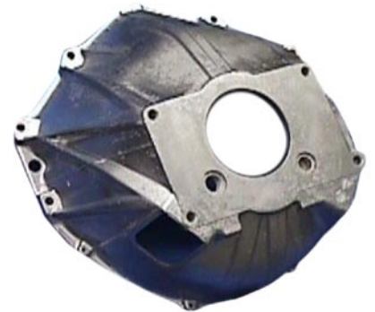
The common transmission pattern as found on most Chevy and many GM bell housings from 1947-1991.
