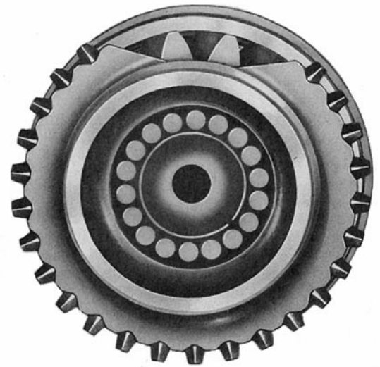
Installing the 18 rollers into the input shaft bore.
