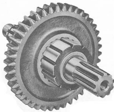
The "skip-tooth" first/reverse gear splines and spline shaft design. Note that we have encountered very rare versions of the 420 that used all 22 splines on the shaft and gear. We recommend replacing this gear with a good used 11 spline version.
