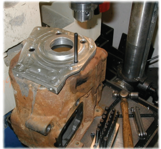
If available, the use of a transfer punch will help start a precise bore.
