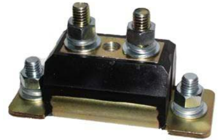
This popular rear mount is what we design our adapters to. It is a common Jeep/Chevy application and well supported by the aftermarket. This one pictured is our favorite, under the Novak #RMU designation.
