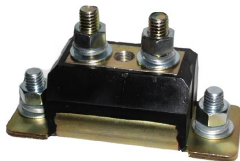
This popular rear mount is what we design our adapters to. It is a common Jeep/Chevy application and well supported by the aftermarket. This one pictured is our favorite, under the Novak #RMU designation.
