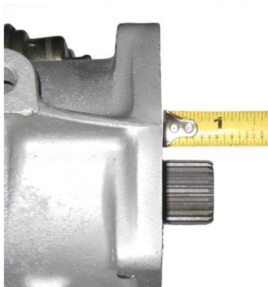
The 4wd version of the TH350 will have a ~3/4" output shaft stickout length.
