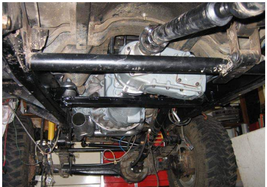
This Jeep featured a hard-mounted adapter, though with isolators at each end of the transmission support crossmember, which offers inferior powertrain flex and unacceptable frame flex. To counteract the latter, the installer welded a tubular crossmember behind the transfer case, which makes future servicing highly problematic.
