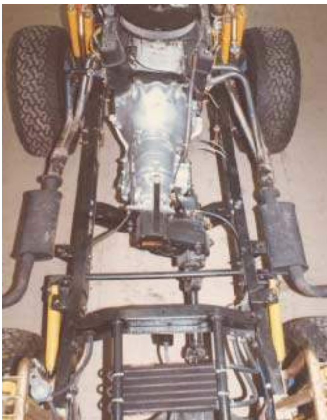
This is a fine installation. The powertrain is offset and parallel to the frame. The Model 18 has a good side mount and the installer has configured an oil cooler at the rear.
