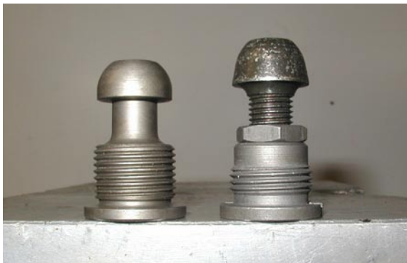
The pivot on the left is a standard GM unit. The pivot on the right is an aftermarket adjustable pivot.
