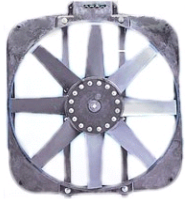
This electric fan is the Black Magic, by Flex-A-Lite. It is one of the best of a new generation of powerful electrics. The included shroud adds to its effectiveness.
