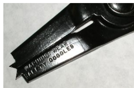
A set of large, bevel tipped, external snap ring pliers is indispensable for removing the large Eaton type retaining rings you'll encounter. These shown are under the Blue Point brand.
