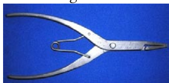
This style of snap ring plier is more universal. With dimpled and knurled flats. They are great for smaller snap rings.
