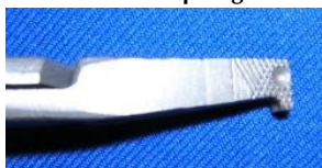
This style of snap ring plier is more universal. With dimpled and knurled flats. They are great for smaller snap rings.
